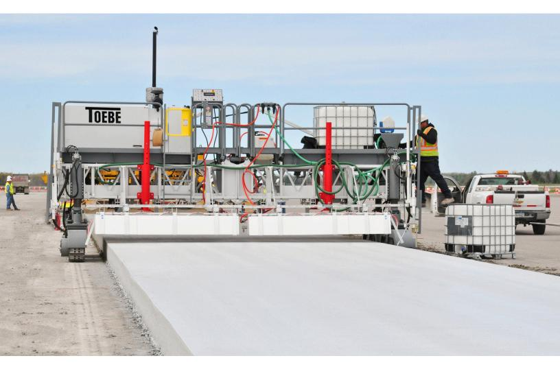
The G&Z TC1500 is the most technologically advanced texture cure machine on the concrete paving market today. The features contributing to this best-in-class distinction include the four-track 90 degree capabilities, the highly accurate steering and elevation control systems, and unique frame design for quick width changes.
